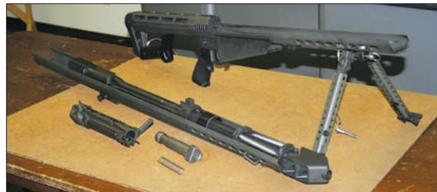
Broken down into its three main components, the lower receiver, upper receiver, and bolt carrier group. Barrett’s simple design is similar to the AR family of rifles.
